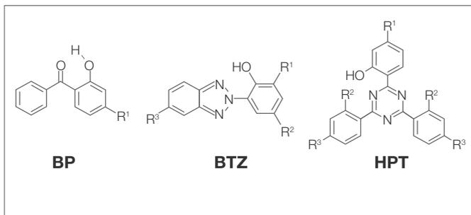
**Fig. 3: Mode of action of 2-(2-hydroxyphenyl)-benzotriazole (BTZ) and 2-hydroxyphenyl-s-triazine (HPT) UV absorbers**
