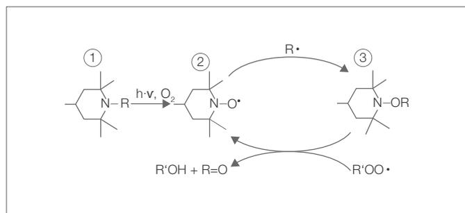
Mode of action of hindered amine light stabilizers (HALS) according to the "Denisov cycle"
